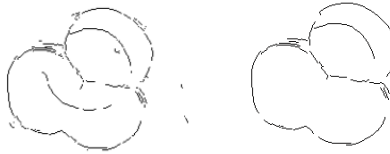
Figure 18: the left image is the boundary detection with the optimal threshold for this image. The right image is the boundary with the threshold for the dataset.
