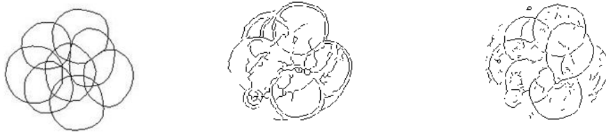
Figure 13: boundary detection results with optimal threshold. The left image is the ground truth, middle one is the edge detection, and the right one is the ridge detection
